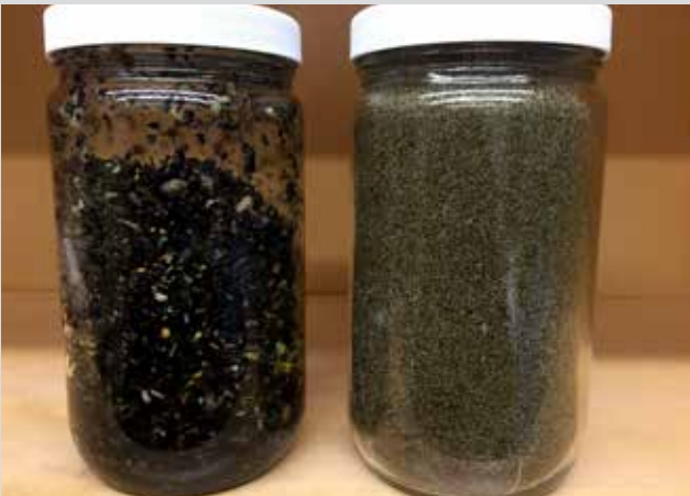
Captured grit from existing removal unit vs. captured grit from pilot removal unit
